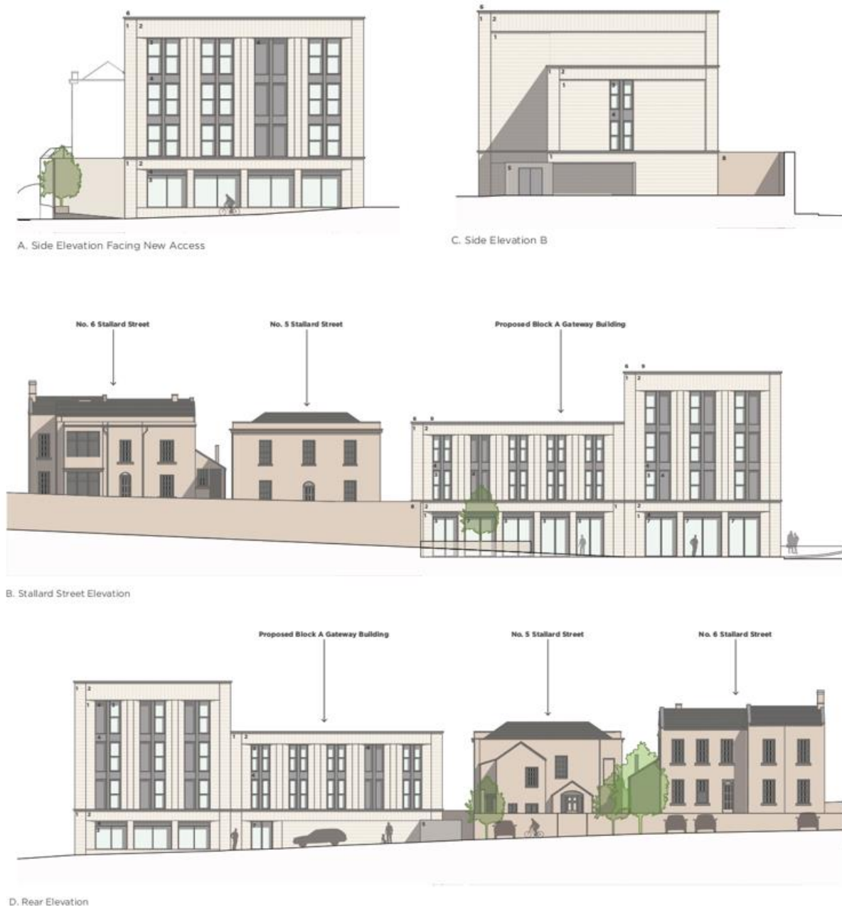
Figure 9 – Gateway Building Elevations
